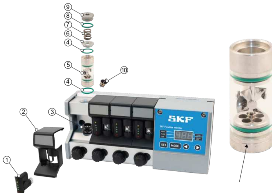
Figure 16 Replacing a flowtube assembly and visible groove
