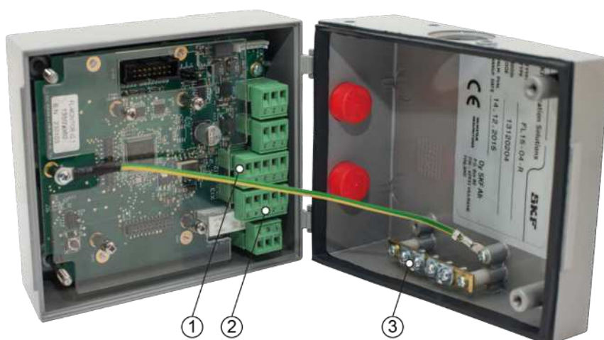
Figure 22 Connectors for CAN bus in monitor, 1: X12, 2: X13, 3: TE-Bar
